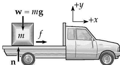
As seen in the free-body diagram of the box given in the sketch, this friction force  $f$  is the resultant horizontal force that will accelerate the box.  $\diamond$
